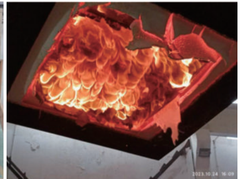
Exposed Surface After Fire Endurance Test ( 120 mins)
