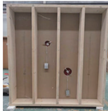
Downlight Install on Ceiling Assembly
