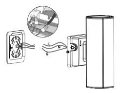
3. Connect the wires: AC/L matches black; AC/N matches white; E matches green.
