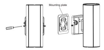
1. Use a tool to loosen the two mounting screws and remove the mounting plate.
