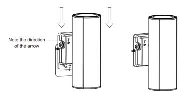
4. Press the upward arrow mark and buckle the lamp from top to bottom onto the mounting plate.
