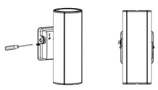
5. Use a tool to tighten the two mounting screws and the installation is complete.
