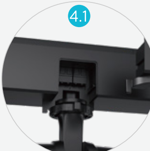
Exchange the whole track adaptor with driver by screwdriver
