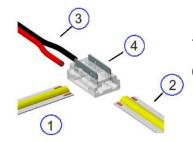
7: Connecting wires to LED strip in T-shape
