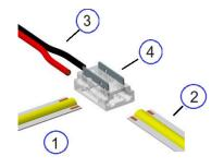
5: Connecting wires to LED strip in L-shape
