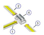
6: Connecting LED strip to LED strip In T-shape
