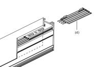
STEP 5 INSTALL THE MSA22 PIN SET(b) INTO THE PIN CONNECTOR HOLES (c) ON THE TRACK. SLIDE THE TRACK CONNECTOR (a) INTO THE SLOT ON THE BACK OF THE TRACK APPROXIMATELY HALFWAY AND SECURE TO TRACK WITH TWO SET SCREWS.
