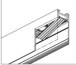
STEP 6 SLIDE MSAS07 TRACK CORNER ONTO THE TRACK CONNECTOR (a) WHILE CAREFULLY LINING UP THE PIN SET ON THE TRACK WITH THE PIN SET HOLES ON THE TRACK CORNER.
