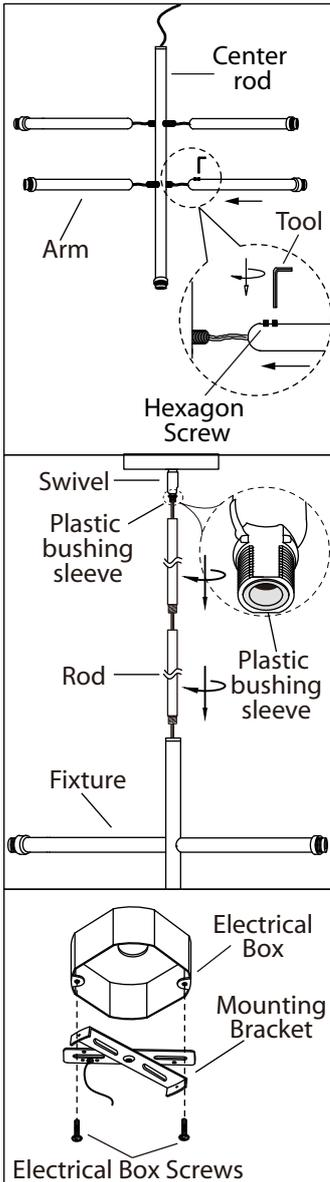
**1.** Screw the arm into the center rod and tighten the 2 hexagon screws by the tool supplied. Repeat this for other arms.
