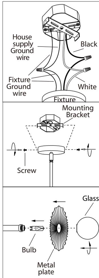
**4.** Connect the ground wires (bare copper or green) from your fixture to the ground wire (bare copper or green) or ground screw in the electrical box. Connect the black wire (or wire with marking) from the fixture to the black wire in the electrical box and connect the white wire from the fixture to the white wire in the electrical box.
