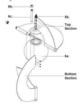
**3.** Attach bottom section to top section with screws **(6a)**, followed by screw cover **(6c)** and secure with finial **(6b)** by threading clockwise
