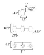
Height from center of autlet to the top of the fixture
