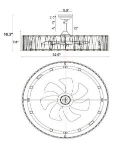
*Note:* The outlet box and Support structure must be securely mounted and capable of reliably supporting a minimum of 50lbs
