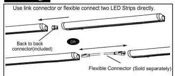
Up to 10 fixtures can be connected with either flexible wire connectors or link connectors.
