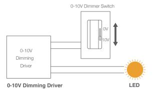
Adjust the brightness of LED light with 0-10V dimmer switch. Slide the dimmer switch to "oV", 4% brightness of LED light. Slide the dimmer switch to "10V", 100% brightness of LED light.
