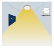
Light dims to stand-by level (10%, 20%, 30% or 50%) if no motion is detected after holdtime.
