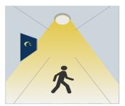
With insufficient ambient brightness, the light turns ON when motion is detected.
