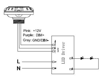
**NOTE:** When both a motion sensor and a 0-10V dimmer are connected to a single luminaire, the brightness of the luminaire will be set to the lowest brightness setting. This applies to output switch settings on power selectable luminaires as well.
