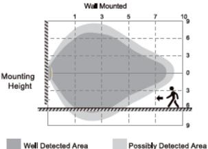
Maximum mounting height is 25ft (7.7m). The figure shows the sensor coverage pattern at the maximum mounting height with 100% sensitivity.
