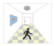
With sufficient ambient brightness, the light remains OFF when motion is detected.
