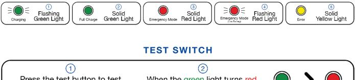
Press the test button to test for normal emergency operation.
