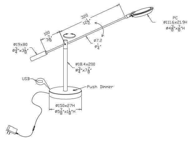
INPUT: AC 100~240V 50/60Hz DUTPUT: DC 24V 500mA
