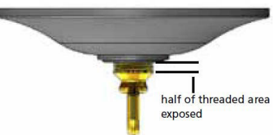
Drawing 2 – Canopy Adjustment
