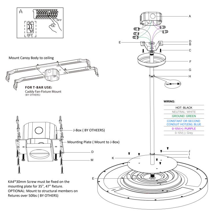
WARNING: Ground fixture in accordance with local and national electriacl codes. Failure to do so may result in serious personal injury.
