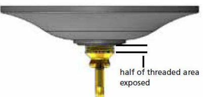
Drawing 2 – Canopy Adjustment
