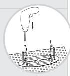
4. Insert the Concrete Anchors (Part C) into those holes and tighten them to the Mounting Bracket (Part B) using the Allen Wrench (Part E).
