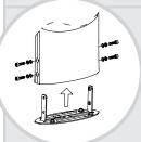
Remove the Mounting Bracket (Part B) from the Solar Pillar (Part A) by removing the four screws and sliding the bracket away from the bottom.
