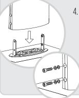
4. Slide the Solar Pillar (Part A) over the Mounting Bracket (Part B) and secure using the four screws (removed from the Pillar earlier) and the Allen Wrench (Part E).
