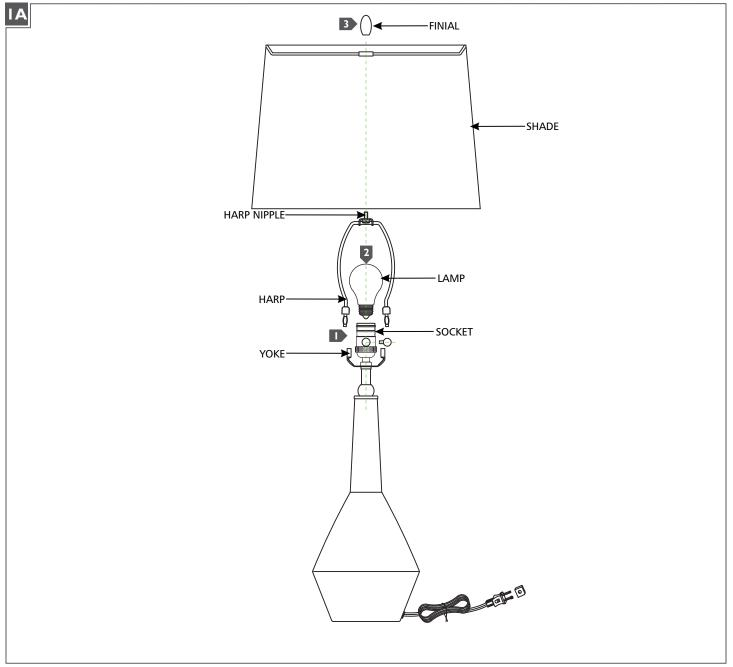
Install the harp by inserting it into the yoke.
