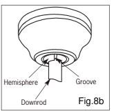
**NOTE:** When installing fan on sloped ceiling, make sure tab on hanger bracket faces towards the top of the slope. Depending on the slope, a longer downrod may be required to prevent fan blades from hitting the ceiling.
