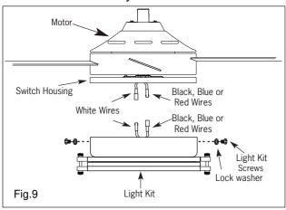
WARNING: Ensure that all connections, set screws and screws are securely tightened before the next step.
