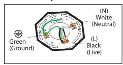
Connect (push) electrical wires from electric box (house wiring) into correct inserts. Black (Live), White (Neutral), Green (Ground)
