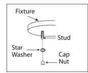
Tuck electrical wires into outlet box and position fixture over studs on mounting bracket assembly. Secure fixture in place with star washer(s) and cap nut(s).
