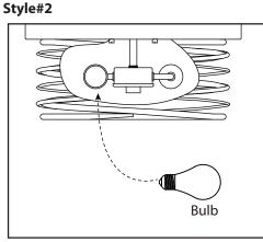
Install specified bulb type and wattage (not included).
