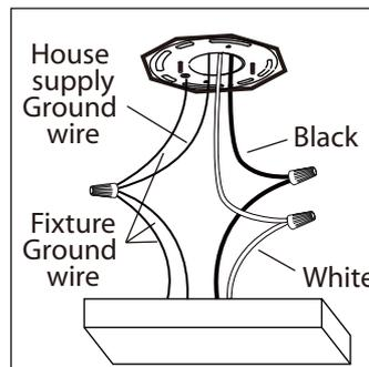
**4.** Connect the ground wires (bare copper or green) from your fixture to the ground wire (bare copper or green) or ground screw in the electrical box. Connect the black wire from the fixture to the black wire in the electrical box and connect the white wire from the fixture to the white wire in the electrical box.
