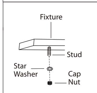
**5.** Once wire connections are completed, carefully tuck wires and wire nuts into the electrical box making sure no bare wire (on the black and white) is visible at the wire nuts. Install the light fixture to the ceiling by aligning the hole(s) in the fixture with the studs on the mounting bracket. Secure fixture in place with star washers and cap nuts.
