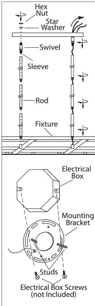
**1.** Install the length of rod that is required by threading wire through the rod and screwing it to the fixture. Install swivel to the rod, ensuring that the sleeve is at the swivel.
