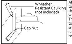
After Installation, seal around the top and side perimeter between the fixture and the wall surface with weather resistant caulking. The bottom should be left un-caulked to prevent moisture build-up. Apply a small amount of weather resistant caulking around the side perimeter between the cap nut and mounting plate.
