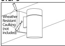
After Installation, seal around the top and side perimeter between the fixture and the wall surface with weather resistant caulking. The bottom should be left un-caulked to prevent moisture build-up. Apply a small amount of weather resistant caulking around the side perimeter between the cap nut and mounting plate.
