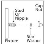
Tuck electrical wires into outlet box and position fixture over studs or nipple on mounting bracket assembly. Secure fixture in place with star washer(s) and cap nut(s).
