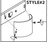
**STYLE#2** - Install proper bulb type and wattage. Install the glass to the fixture by tightening the 2 thumb screws.
