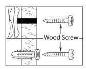
Additional support may be required for fixtures longer than 20". Position the fixture and add wood screws (one on each side) for the wooden studs or plastic wall anchor and wood screws for dry wall.
