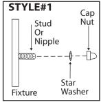
**STYLE#1**-Tuck electrical wires into outlet box and position fixture over studs or nipple on mounting bracket assembly. Secure fixture in place with star washer(s) and cap nut(s).
