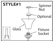
**STYLE#1** - Remove spinner nut from socket. Position glass on the fixture and secure with spinner nut. Install proper bulb type and wattage. **Note:** Glass may face up or down.
