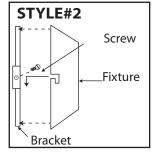
**STYLE #2** - Insert one screw into the mounting bracket - do not tighten yet. Tuck electrical wires into outlet box and position fixture over the mounting bracket. Line up the screw in the bracket to the "7" hole on the fixture. Slide fixture to secure in place. Insert remaining screw. Tighten both screws to secure.
