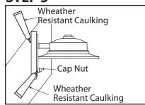
After Installation, seal around the top and side perimeter between the fixture and the wall surface with weather resistant caulking. The bottom should be left un-caulked to prevent moisture build-up. Apply a small amount of weather resistant caulking around the side perimeter between the cap nut and mounting plate.
