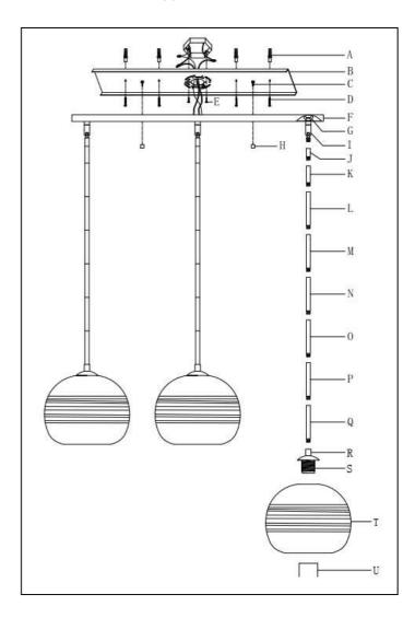
Line art shown may not exactly match the fixture enclosed. However, the installations do apply to this fixture. ITEM NO: 486P10-3L
