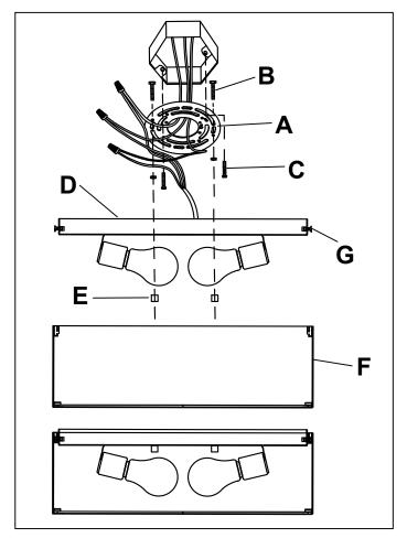
Line art shown may not exactly match the fixture enclosed. However, the installations do apply to this fixture. ITEM NO: 2302-F1,2302-F2,2302-F3,2302-F4 2303-F1,2303-F2,2303-F3,2303-F4
