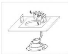
Bypass ballast & wire to j-box
