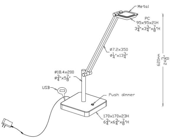
INPUT: AC 100~240V 50/60Hz DUTPUT: DC 24V 500mA
